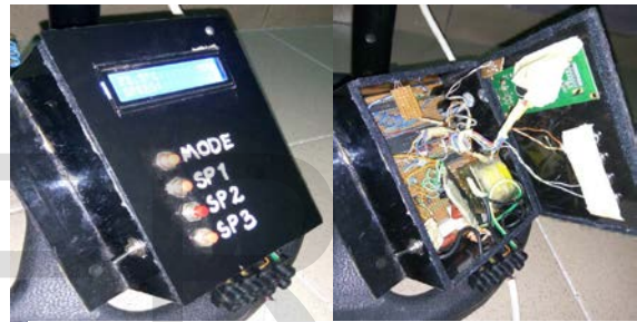
The Receiver Fan Regulator packaged in PVC
