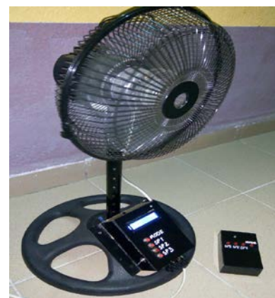
Figure 9: The complete Temperature-controlled Smart Fan System with Remote Control Unit
