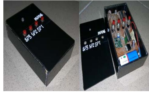
Figure 7: The packaged Remote Control unit (Transmitter)
